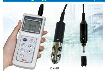
Oxygen which is passed through Diaphragm in the Oxygen Battery Tank, is resolved at the Cathode and resolved Electric Current in proportion to Oxygen Density flows between Anode and Cathode.
